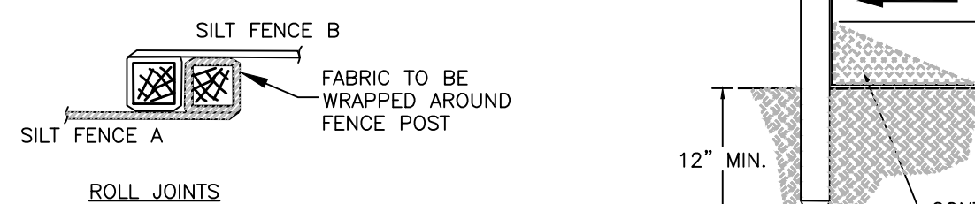
1 SILT FENCE INSTALLATION DETAILS C300 NOT TO SCALE
